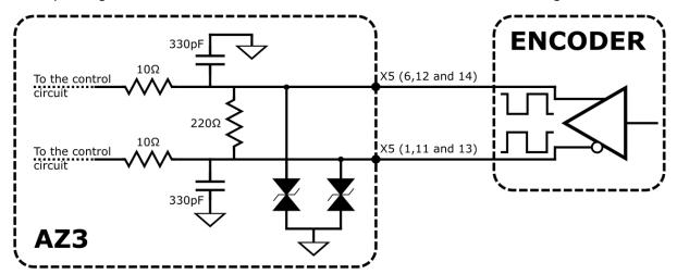
The input stage schematic of channels of Hall encoder is showed in the image below:
