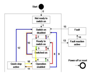
Operation enable is the only state in which the power stage is enabled.
